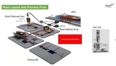
The plant is an integrated steel plant. JSIS have 2 MTPA DRI plants (Technology by Midrex) which is directly connected with SMS (EAF) and 2.4 MTPA (Technology by Danieli). After SMS, they have 1.5 MTPA rebar rolling mill with hot charging (Technology by Danieli). There is one EAF furnace of 36 MVA for SiMn which daily production will be 150 MT/ day and 4500 MT /month.
