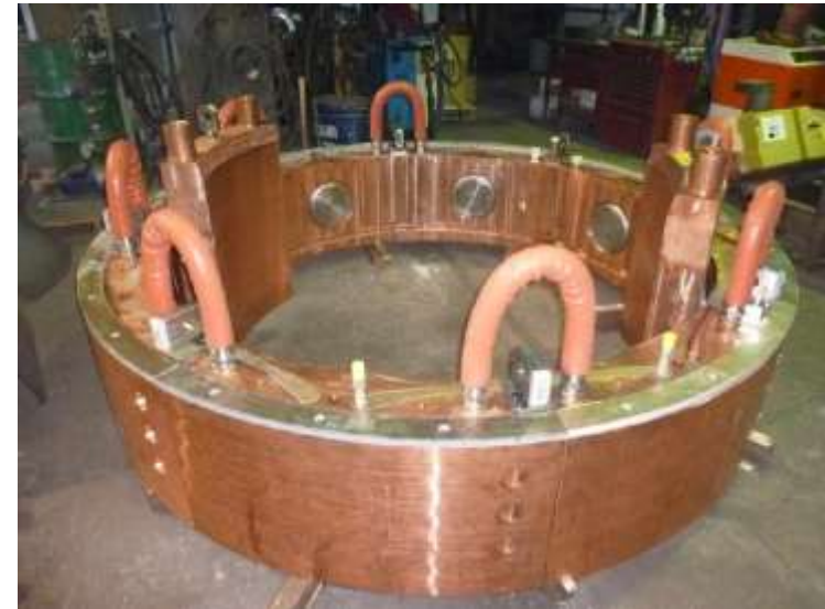
Electrode bottom components - trial assembly in France and South Africa.
