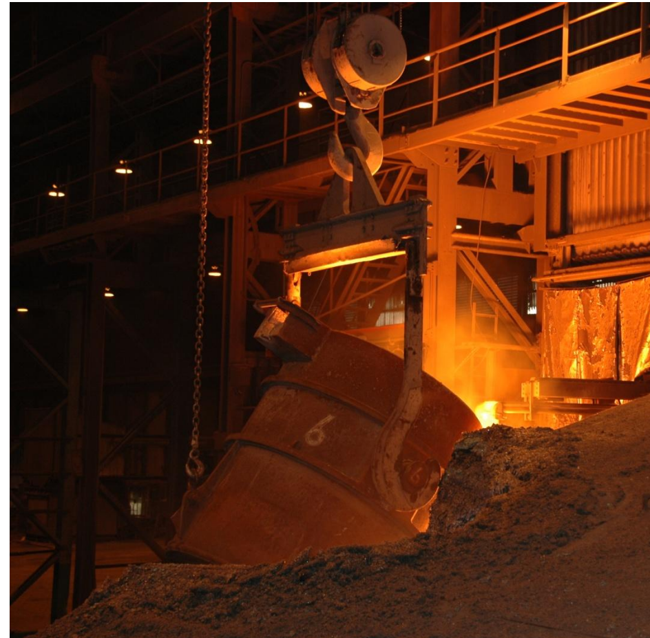
Protective “skirts” during foaming of the ladle.
