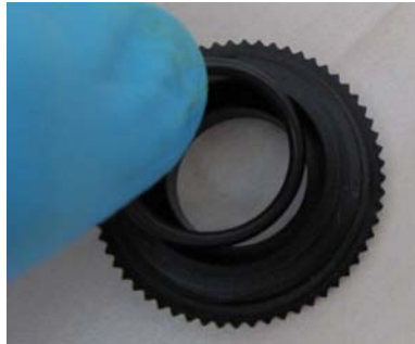
Figure 5 Placement of the O-ring B inside the inner recess of the front plate of the IOM sampler
