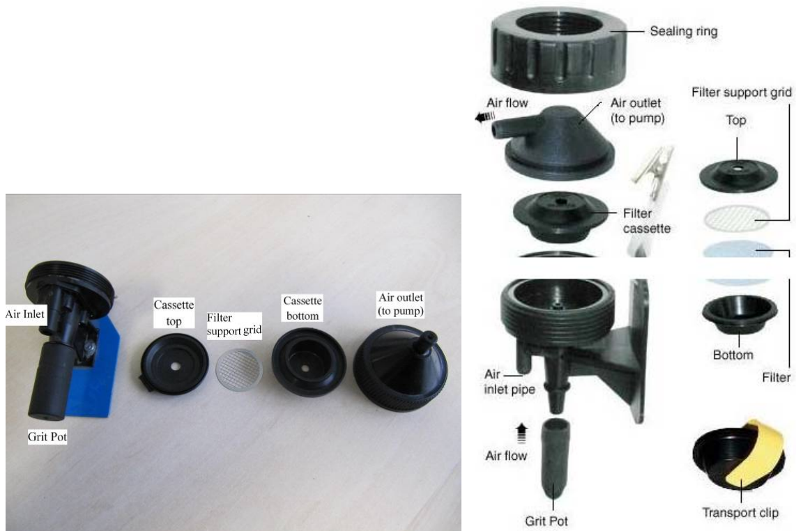
Figure 9 SKC plastic cyclone components (left) and Casella Measurement plastic cyclone components (right)
