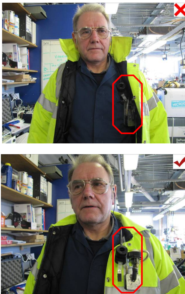
Figure 12 Simultaneous sampling with the HD cyclone and IOM head. Wrong collocation with jacket covering one of the samplers (top) and right collocation (bottom)
