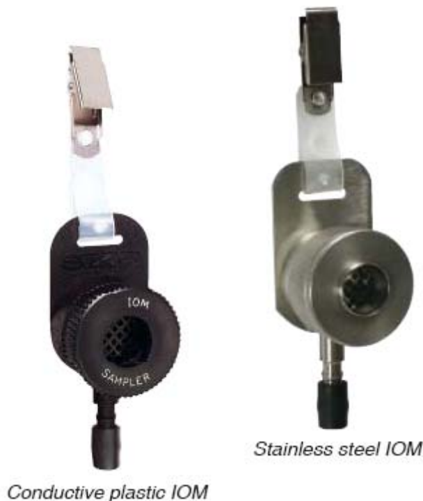
Figure 1 IOM conductive plastic (left) and stainless steel (right) sampler (source: http://www.skcinc.com/instructions/37372.pdf )
