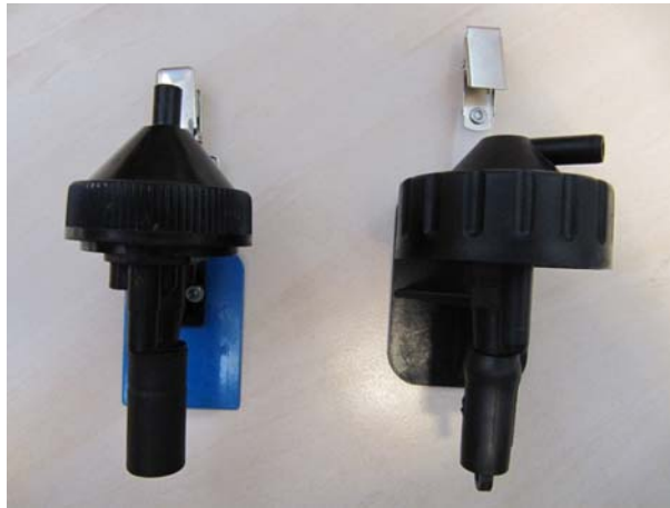
Figure 8 SKC Higgins Dewell (HD) cyclone (left) and Casella Measurement HD cyclone (right)
