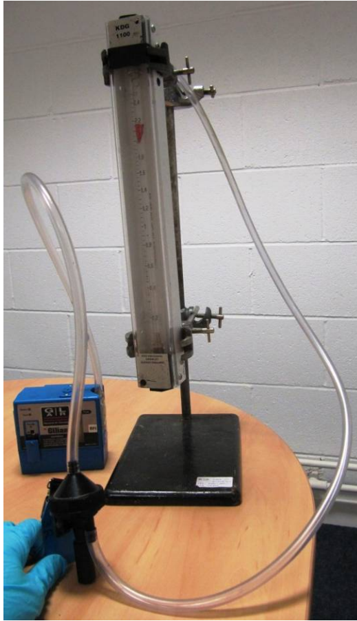
Figure 11 Calibration of the HD SKC cyclone using a rotameter
