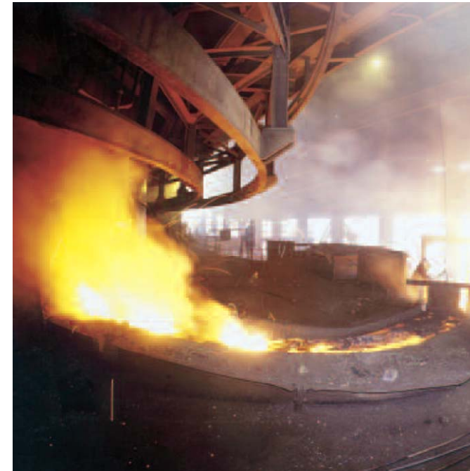
Casting of ferro-manganese from a smelter furnace
